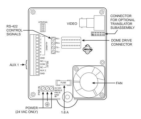
Figure 12. Interconnect Circuit Board Electrical Connections for Spectra II™
